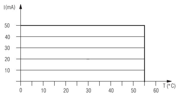
Quadratic total current limit curve semiconductor monitoring outputs
