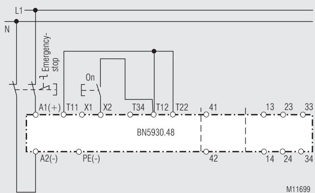
Two-pole emergency-stop with emergency-stop control device in the supply circuit..
