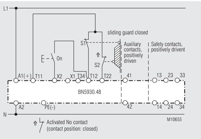
Two-channel monitoring of a safety gate.
