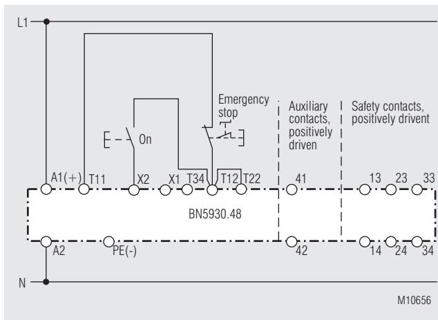
One-channel emergency-stop circuit. This circuit does not have any redundancy in the emergency-stop control circuit.
