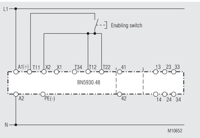
Emergency stop circuit with control of enabling switch.
