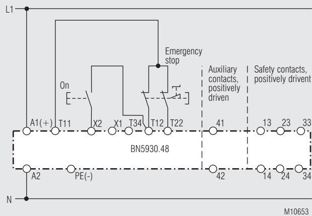
Two-channel emergency stop circuit
