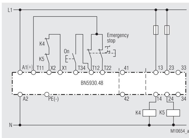
Contact reinforcement by external contactors, 2-channel.
